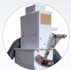
Highly Efficient Pneumatic Sheller/ Dehusker used for separating husk from brown rice
