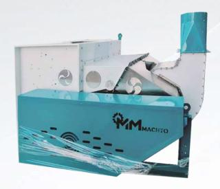
In the rice milling industry, Husk Aspirator plays a crucial role in ensuring the rice we get is clean and high-quality. They focus on removing the husk from the rice grain using airflow to separate the husk from the rice gently. This helps in getting cleaner rice and contributes to making the entire rice milling process more efficient.
