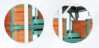
Highly Efficient Rice Shifter is used to grade grains based on size.
